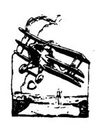
Our model packs 90 square inches of wing area into a mere 16 inch span allowing it to be almost completely structured with 4 to six pound 1/16 square balsa thus achieving a very low wing loading. The completed model weighs 1.1 ounces complete with motor and ballast.
