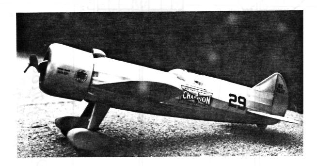
Lookin' as clean as a whistle, Mark Fineman's Thompson entry was scratched from the list when her gear was damaged in a hot landing during the Shell. This Pesco Special was built over Cleveland plans with considerable simplification to lighten the wing loading. All of you pylon polishers will have to contend with this bird again, come spring!
