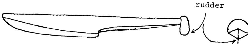
Usual float for model aircraft. Internal keel (crutch) large rudder.
