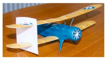
At this point, the wings will still have enough spring in them to allow the later addition of the hard balsa interplane struts, though it is best to slip the jig over the wings again once you have done this to recheck the angle and spacing.
