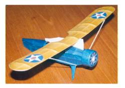
You now have a sort of parasol arrangement, which will be rigid enough to stay in place while you add the four center section struts one at a time. The model plan calls for 1/16" sq. balsa for these, but I used "cocktail" sticks for strength. These had been previously covered in blue tissue, to match the fuselage, and were attached using cyano glue.
