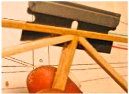
Now to the cutting apart. The only places the box sides stick together are at the glued joints. You can slip a razor between the sticks at any other place, and push toward the joined spot and it'll cut/crack loose. Takes about five minutes to do the whole thing. A very important thing first, when you are ready to separate the sides, mark an "X" on the front or back of the whole frame to remind yourself which are the OUT-sides. You'll need this little nicety just once, but it's a big once.
