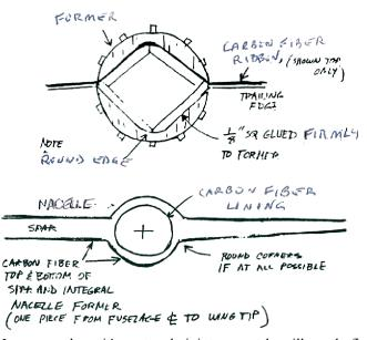
In cases where it's a tough joint, a patch will work fine although at a weight increase. .
