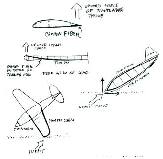
A strip of CF inside the outline of a vertical stab would protect it during a hit-the-nose-flop-over-on-the-back landing. Same thing would apply to horizontal stabs., Even just a strip along the central stabilizer spar may be enough.
