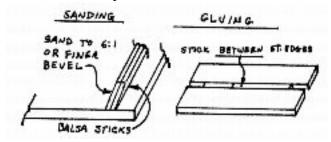
Have you ever had a crack in a sheet balsa part on a plane and wanted to glue it? If you can get to the edge of the crack, carefully spread it apart. On both sides of a piece of bond paper about as wide as the crack is long, put a bead of white glue on both sides. Work the paper into the crack and let it close on the glue, open the crack a little and work the glue around, then remove the paper. As the crack closes, you will find that the crack is well and truly glued.
