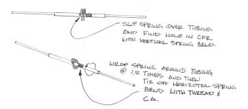
The critical decision you've got to make when you mount this system in the fuselage is that you've have to make sure the slot in the aluminum tubing is facing the correct direction and at the correct at the angle you wish to have the stab be rotated to. The slot, in effect is the stop for the stab rotation.
