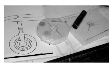
Using a draftsman's compass centered on the hole you just drilled in the balsa plug, draw a circle on the foam blank slightly larger than the finished wheel. Rough cut the foam
