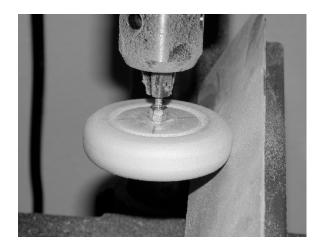
After sanding the outer tire to the correct diameter and rounding it, use a small jeweler's file to cut the inner tire rim, and if you want tread, now's the time to use the same file to create the tread. If the "metal" part of the wheel has a conical profile, a small stick with sandpaper will come in handy to create that.
