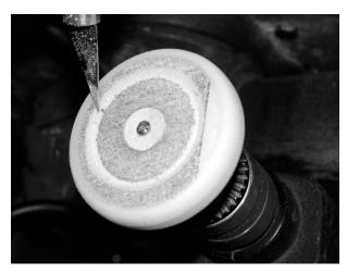
Paint it first with thinned Elmer's glue, sand, and then paint with cheap artist's water based acrylics. I mixed some red in with the black to get the black closer to what a rubber tire would be. Cut out a paper wheel/rim and glue it on with foam friendly glue.
