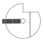
Whichever technique you use, unless you enjoy hearing the exciting sound of a rubber motor rekitting your model, you should ensure that you've filed a flat spot on the prop shaft to hold the set screw.
