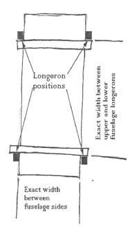
Make a cross piece which is installed to separate the two parts. This separator is glued between the vertical jig plates using CYA or white glue after they have been attached to the fuselage sides with rubber bands.
