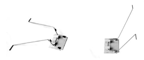
I've since learned that there is no need for a slot to hold the rear of the gear wire. In fact a quartering downwind landing will tend to break the slot. A simple piece to prevent the gear from shifting aft is enough. I've also learned that the 1/8"X1/16" magnets hold the gear just as well, and that it is possible to accomplish this set-up with less weight than that shown here.
