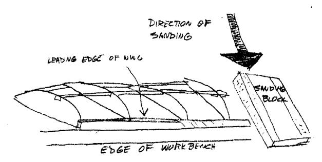
Good way to shape wing leading edge is to put at edge of bench and "wipe" your sanding block downwards. Always use fresh sandpaper and let it do the cutting, not your hand pressure.
