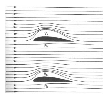
If the gap is small, this interaction results in a considerable loss of lift. In the case of the triplane airflow shown below, the middle wing is affected most because both pressure under and vacuum over that wing is reduced.
