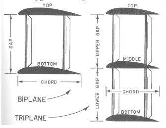
In spite of the previous statement, Grant suggests a gap equal 1-1/2 times the chord for models. He cautions to never use a gap less than one times the chord, nor more than three times, for there is no advantage in doing so.
