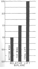
**Triplanes.** The lift and efficiency of a triplane is even less than that of a biplane. Grant advises using a gap of not less than 3/4 nor no more than 1-1/2 times the chord. Of course the larger the gap, the greater the relative lift and efficiency. The following tables show the relative lift and efficiency of monoplane, biplane and triplane models at various angles of attack with a gap of 1-1/4 times the chord, again assuming the same chord.
