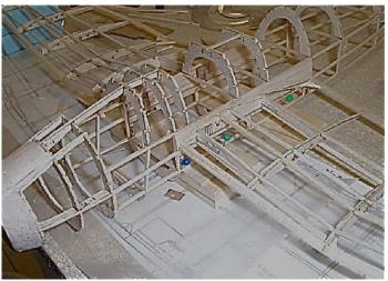
Gene used a combination of 1/16" and 3/32" tubing for the rear spars and 3/32" and 1/8" tubing for the main spars. **The larger tube in each pair is mounted in the wing, with the smaller tube attached to the fuselage.** When doubling the wire for the T, it should be a snug fit inside the smaller tubing. Gene used .025" wire for the 3/32" tubing and .015" wire for the 1/16" tubing.
