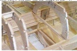
Each of these "Ts" are mounted on a piece of 1/64" ply which will be epoxied into the fuselage as shown in the photo above. The wire "Ts" are epoxied into a piece of aluminum tubing about an inch long, which will telescope into other aluminum tubes mounted between spars in the wing. The wing tubes may be seen in the photo below.
