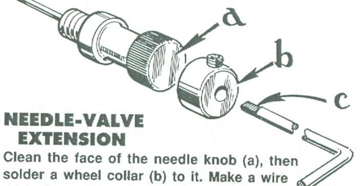
solder a wheel collar (b) to it. Make a wire extension, and file a flat (c) on the end to allow it to be properly gripped by the wheel collar's setscrews. When the engine is switched between models, this setup allows the use of extensions of various lengths.
