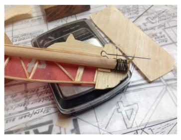
Fifth, build and assemble the landing gear. Because so much weight was going to be need to balance the plane in the correct location, very little effort was made to keep the weight out of the wheels, so much to the point that the centers of the wheels were thickened up to allow a propeller bearings to be used to ensure the wheels would roll freely and smoothly.
