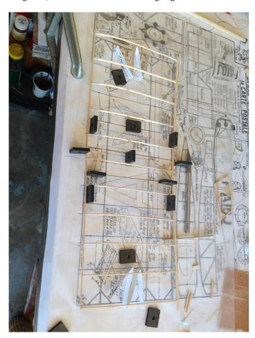
**First, build the wing.** The shape of the wing's airfoil was transferred to a piece of 1/16-inch thick stock, it was cut, waxed and pinned to a board. With the airfoil template done, the 22 pieces needed for the 11 ribs, 1/16-inch square, were cut out. They were curved by using a rolling motion of an x-acto blade handle to compressing the wood on a hard surface. Two of these pieces
