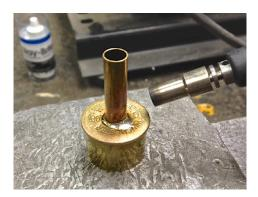
Put some good solder flux on the joint between the tube and the shell, being careful not to disturb the alignment, heat the junction very hot with a torch and touch with solder and you've got yourself a tool for cutting nose plugs as shown in Wally's article.
