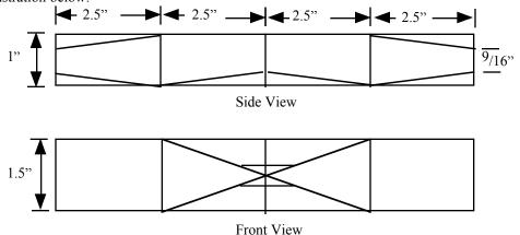
Once we finish these calculations we move into the world of folklore. The width of the block where the prop shaft goes through is normally between 3/8" and 1/2", and the fore and aft thickness of the hub is normally in the range of 5/8 to 3/4 X the max thickness of the prop block.
