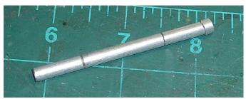
I always reinforce the motor peg holes in the fuselage with a piece of 1/64" ply which has been hardened with thin CA, so that the peg assembly fits snugly in the fuselage and won't become a sloppy fit with use. Based on advice of some older boys, I CA'd onto one end of the assembly a short ring of aluminum tubing of still the next larger size than the rest of the assembly. I've found that when inserting the motor peg
