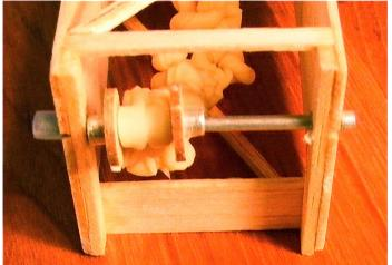
The critical part of Stew's scheme is to cut a short piece of aluminum tubing, at least two sizes larger than the motor peg.
