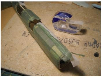
Once the glue is dry, carefully peel the tape back on itself and you have a nice clean line right to the edge of the stringer. If there's a bit of fuzz left, just wet it down with glue and you're home free
