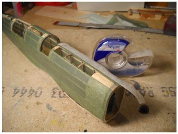
Tom uses thinned white glue to attach his tissue, so in these photos he attaches the last strip of tissue to one stringer of the open bay without the use of the tape. He said the smart move would be to use tape on both stringers, but he found the job of cutting the tissue straight to fit one stringer was easy enough so he didn't use the tape on that one. As ham fisted as I am with tissue, I would have used the tape on both stringers.
