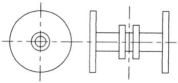
The bobbin can easily be made from either sheet plastic or 1/32 ply disks CA'd or epoxied to a piece of aluminum tubing. The spacing of the inner rings should be equal to the
