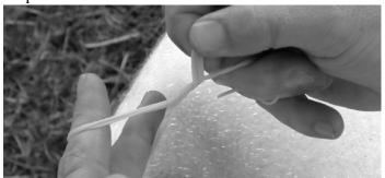
Step 3. While keeping your two fingers spreading the loop, reach your thumb through the loop and grab both ends of the broken strand, keeping the rest of the motor in your right hand. Pull the broken strands of the broken motor through the loop.
