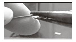
Step 1. Start with a wire that is much longer than what is needed for the prop shaft. It can be cut down to size later. Grip the wire with the tip of the pliers about 1 inch from one end of the wire.
