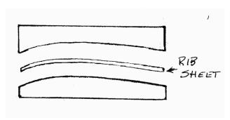
Then, sandwich the sheet between the two halves of the form, with the desired rib width extruding to one side. Using a fine tooth hobby saw, slice the ribs one at a time. You can then glue a straight piece under each rib to form the rib bottom either before or after you set the spar in place.
