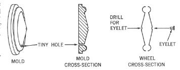
This subterfuge makes use of a Mattel Vac-U-Form toy to mold the wheel and tire in halves, from clear plastic sheet.
