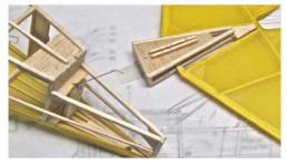
The spring which kicks up the stab is made from .015 music wire, shaped as below. The zig zag portion is sandwiched between to sheets of balsa with Duco and fixed to a bulkhead below the forward edge of the stab.
