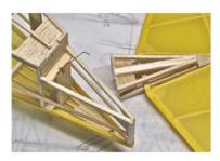
The top of the stab (shown above) is also sheeted and a nylon hinge (difficult to see in these photos) found in RC model supply houses is used to attach the tail assembly to the fuselage. A 1/8X1/16 stick is installed as a base for the rudder. Also visible in the photo is a hole in the bottom of the fuselage through which the pull-down line will be run. The same setup leading to the button timer is used here as discussed above.
