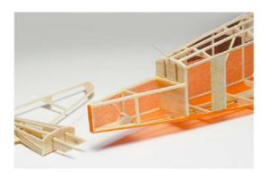
You'll notice that Tom, a man with "class," keeps his pull-down line inside the fuselage until shortly before it reaches the button timer. The use of a soda straw to shield it from the flailing rubber motor would seem a worthwhile thing to do.
