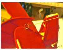
A very short piece of 1/8 aluminum tubing was crimped onto the pull-down line to act as a stop to prevent the entire tail from tilting forward more than 45°. It hits another short piece of 1/8 tube CA'd to a bottom longeron, through which the pull-down line runs. The crimped tubing and the CA'd tubing can be seen in the following photo.
