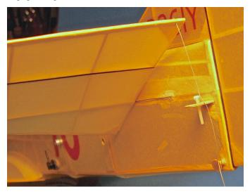
He simply used a single hole paper punch to make a round piece of 1/64 ply which he glued to a short piece of round toothpick, CA'd into a reinforced part of the stem post of the airplane. Works like a charm.
