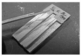
To use this, you place the un-rounded strut between the guides flush with the end of the notch in the plywood. Hold the strut in place with your thumb and run the saw flush on the plywood across the strut. The stiffening rib on the saw will prevent it from going in too deep and you get a nice centered cut in the end of the strut 1/8" deep. Since I am using a very fine 52 tpi 4-1/2 inches Long x 13/32 inch Wide x .008 inch thick saw the slot is not quite thick enough for
