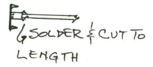
After soldering, Bill inserts the tube and blind nut into the noseblock, then takes a pin and punches a series of small holes in the nose block close to the blind nut, and soaks the area with thin CA. He recommends extending the brass tubing aft of the nose block by about 1/16 inch and soaking the area around it with thin CA, being careful not to allow any CA into the tube.
