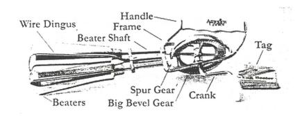
The first pic is of an eggbeater as found in WalMarts, dewy eyed and fresh from China. The second is what happened to the poor thing. Note the construction - - with the Beaters held in place by the Frame and Spur Gears. The following won't work on the kind of eggbeater where the Wire Dingus holds on the Beaters.
