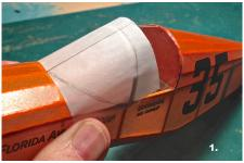
Then clean up the lines using a French curve (2). By folding the tracing paper along the straight line you can then duplicate the lines on the first half, thus producing a nice, symmetrical pattern.
