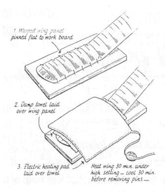
Jack Brombly, Lancaster, Calif., recommends use of damp towel and heating pad for straightening warped wings. Important to leave wing pinned in place for half hour after steaming, says Jack.
