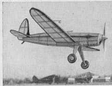
No. M2 Senior Dart 24 in. This low-wing model, with a movable wing for balance adjustment, is very easy to fly. Kit includes pilot and spinner.
