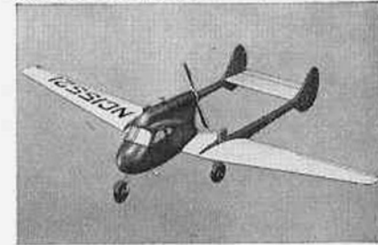
No. J13 Stearman Hammond 10 in. Menasco powered U. S. Government developed safety plane of all-metal construction with fabric covered wings.
