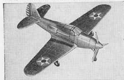
No. J10 Bell Airacobra 9 in. Has 1000 HP. engine mounted behind pilot and cannon firing thru prop hub. Does over 400 M.P.H.
